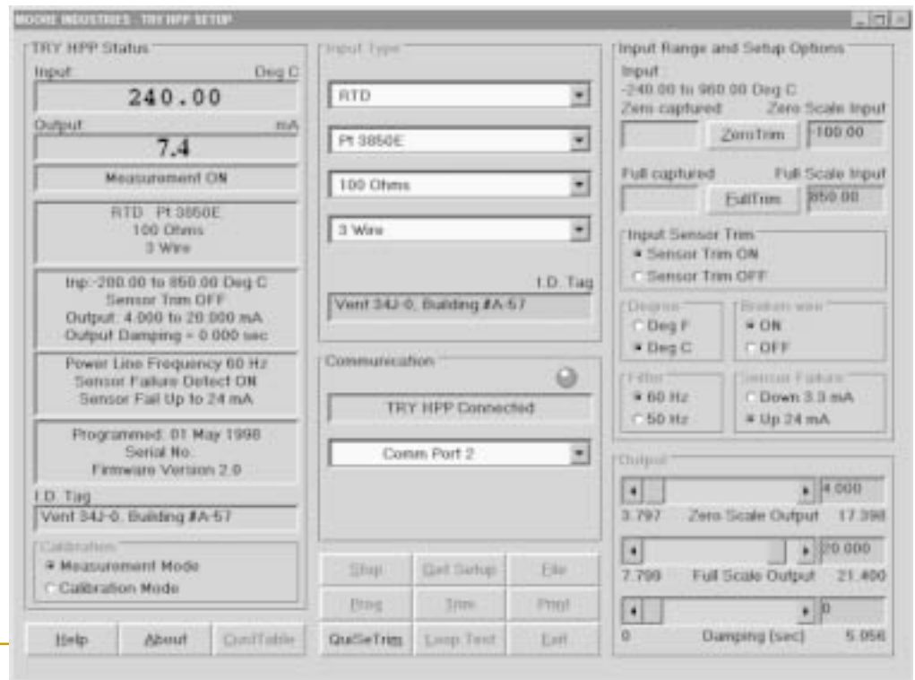
Figure 4. All operating parameters can be set, and then viewed, on a single software screen.
